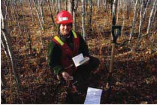
Soil samples are taken at each 5 hectare plot throughout the woodlot inventory
